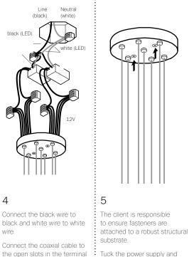
Tuck the power supply and wiring into the canopy. Line up the fastener holes or connect directly to structural ceiling surface using the fasteners
